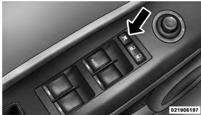
Window Lockout Switch
