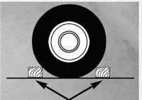
Block both the front and rear of the wheel diagonally opposite of the jacking position.
