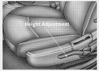
The height adjustment control lever is located on the outboard side of the seat.
