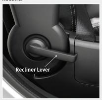
Lift the recliner lever located on the outboard side of the seat, lean back and release at the desired position.
