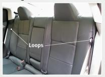
To fold the rear seatback forward, pull on the loops to fold down either or both seatbacks. When returning the rear seatback to the upright position, be sure the seatback is latched.
