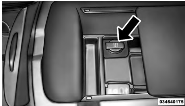
Center Console Power Outlet
