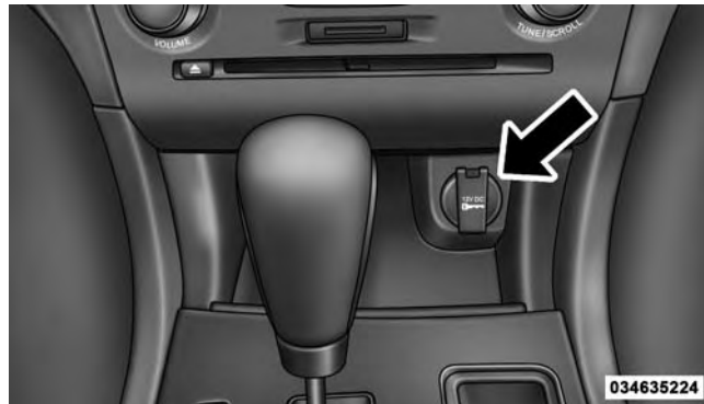
Front Power Outlet
