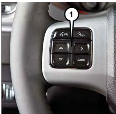
1 – Electronic Vehicle Information Center (EVIC) Controls
