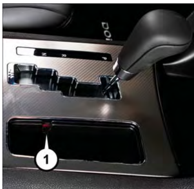
1 – Shift Lever Override Access Port
