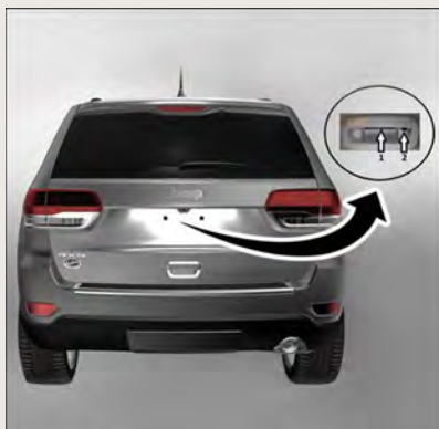
Electronic Release Switch Location
