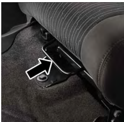
Adjusting Bar Location
