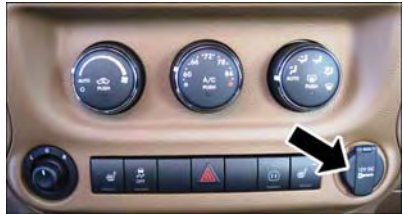
Power Outlet — Front
