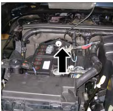
Positive Battery Post
