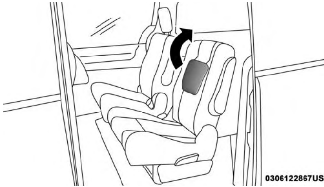
Raising The Head Restraint
