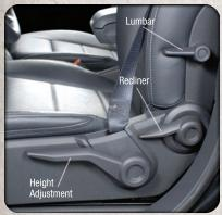
• Lift the recliner handle located on the outboard side of the seat, lean back and release at the desired position.
