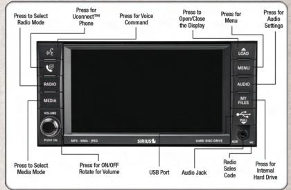
**NOTE:** Your radio may not be equipped with the Uconnect<sup>™</sup> Voice Command and Uconnect<sup>™</sup> Phone features. To determine if your radio has these features, press the Voice Command button on the radio. You will hear a voice prompt if you have the feature, or see a message on the radio stating "Uconnect Phone not available" if you do not.
