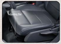
• Lift up on the adjusting bar located at the front of the seat near the floor and release at the desired position.
