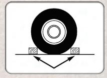
Block both the front and rear of the wheel diagonally opposite of the jacking position. For example, if changing the right front tire, block the left rear wheel.
