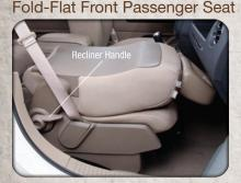
The front passenger seat can be folded flat. Pull up on the recliner handle, to the full upward position, to fold down the seatback.
