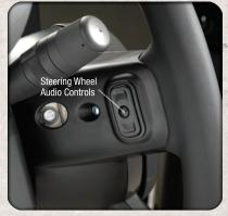
The steering wheel audio controls are located on the rear surface of the steering wheel.
