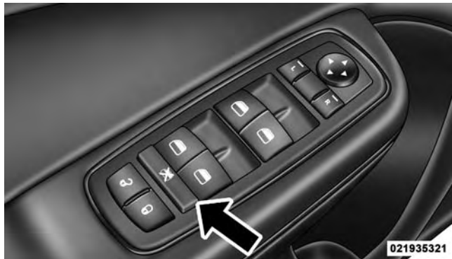
Window Lockout Switch
