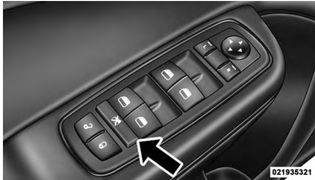
Window Lockout Switch
