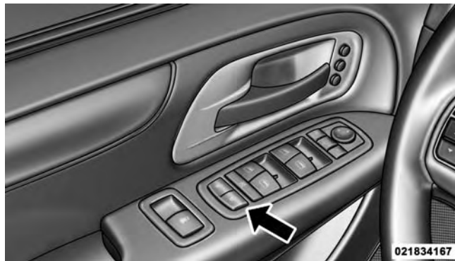
Driver Power Door Lock Switches
