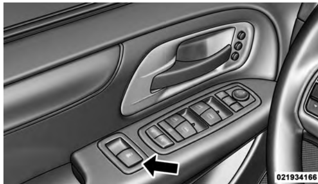
Power Vent Window Switch Open/Close
