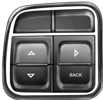
EVIC Steering Wheel Buttons
