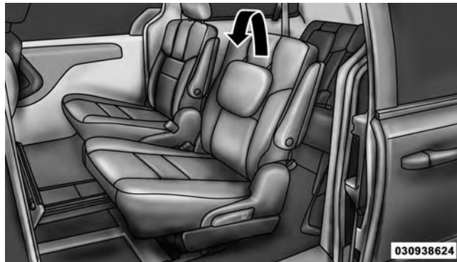
Non-Adjustable Head Restraint
