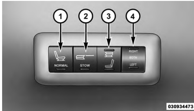
Rear Panel Power Switch Bank
