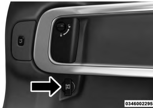
Rear Electrical Power Outlet
