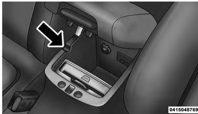
Center Console USB/AUX Connector Port Cable Routing
