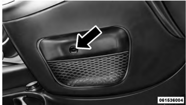
Shift Lever Override Access Hole
