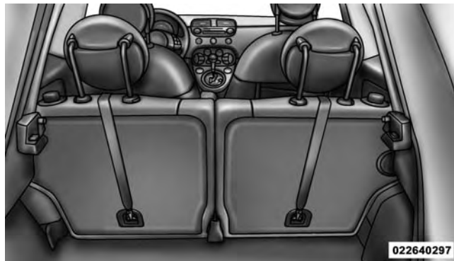
Rear Seat Tether Strap Mounting
