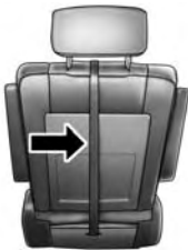
Rear Seat Tether Strap Mounting (Second Row Anchorage Shown)
