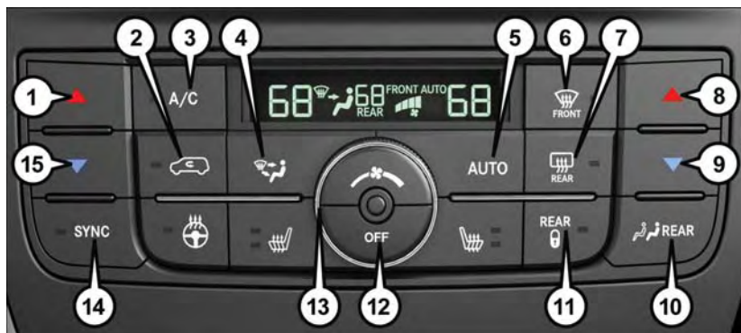
Three Zone Automatic Temperature Controls (ATC)
