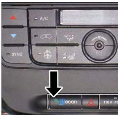
ECON Switch Location
