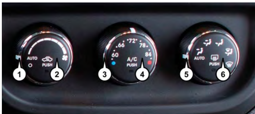
Automatic Temperature Controls
