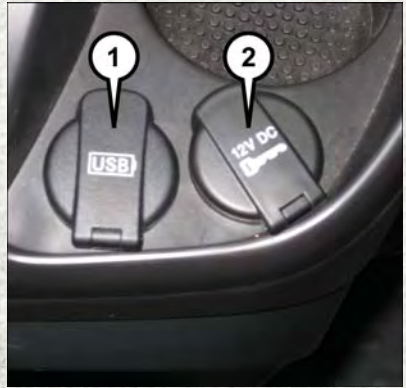
Front Power Outlet
