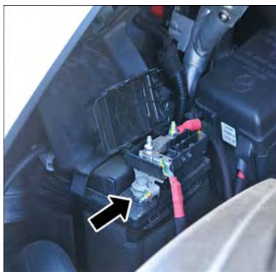
Positive (+) Battery Post
