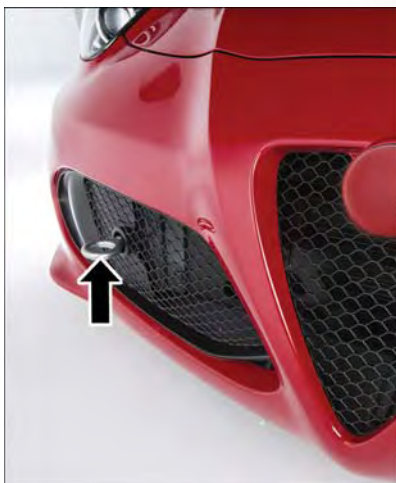
Front Tow Eye Installed
