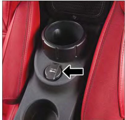
Rear Power Outlet
