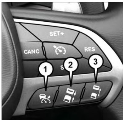
Adaptive Cruise Switches
