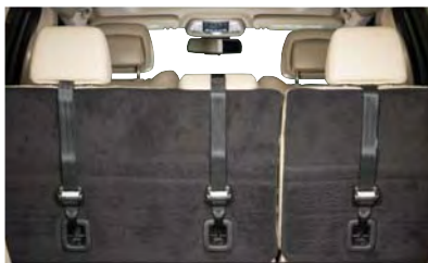
Top Tether Strap Mounting (60/40 Seat)
