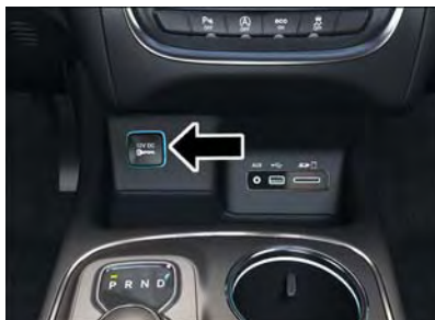
Front Power Outlet
