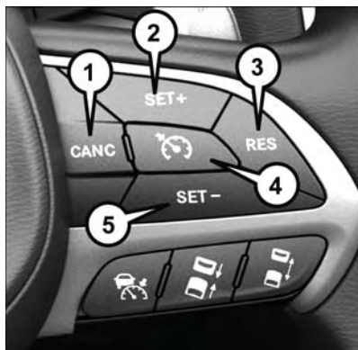
Electronic Speed Control Switches
