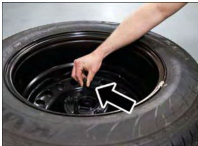
Protective Plate Removal
