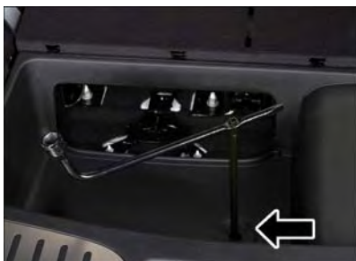
Winch Drive Nut Location
