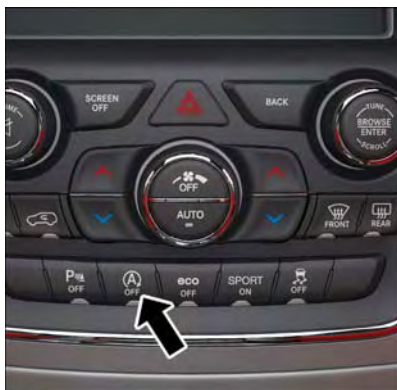
STOP/START Off Switch
