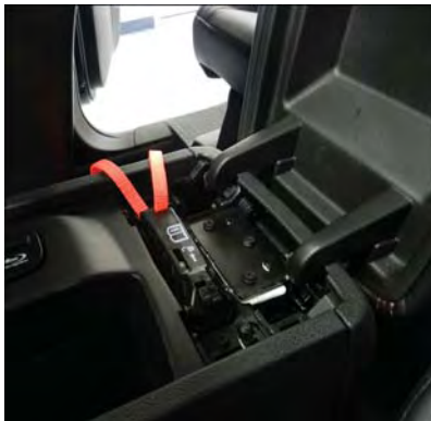
Manual Park Release Cover Removed
