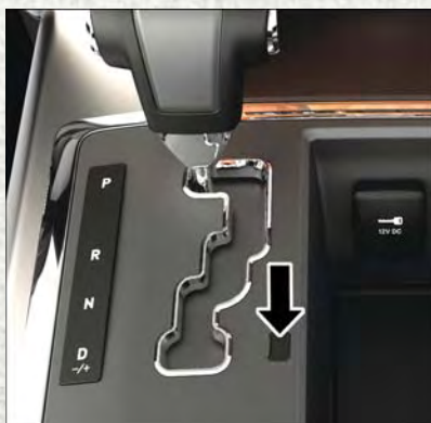
Shift Lever Override Access Cover
