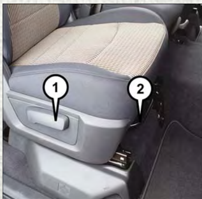
Manual Seat Adjusting Bar/Recline Lever
