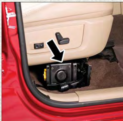
Jack And Tool Bracket Assembly
