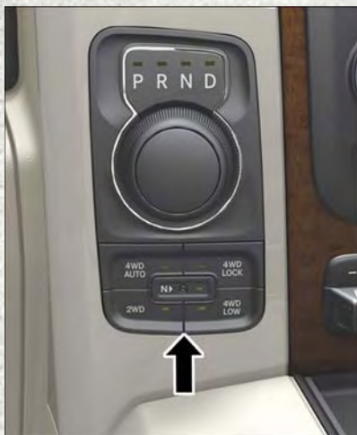
Five-Position/On-Demand Transfer Case — Eight Speed Transmission Only
