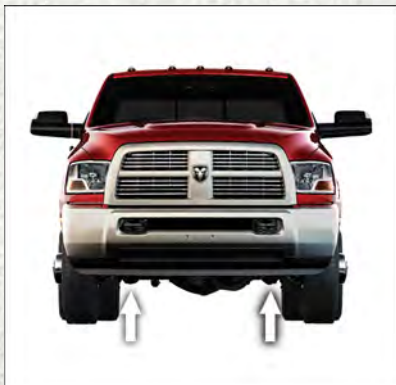
Front Jacking Location
