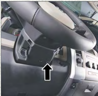
Shift Lock Manual Override Access Port
