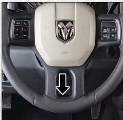
Hood Release Lever Location
