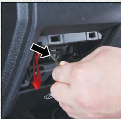
Manual Park Release Lever Locking Tab
