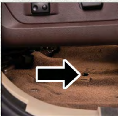
Floor Fastener Location
