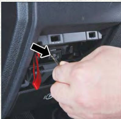
Manual Park Release Lever Locking Tab
