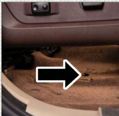
Floor Fastener Location
