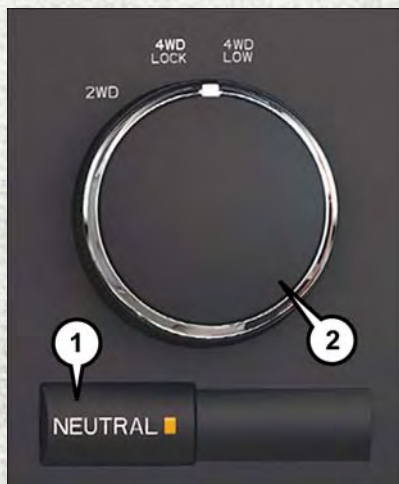
Four-Position/Part Time Transfer Case
