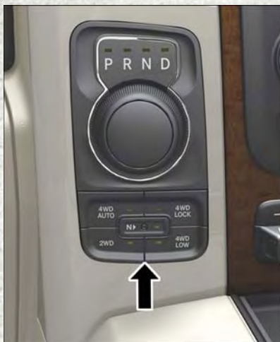
Five-Position/On-Demand Transfer Case — Eight Speed Transmission Only
