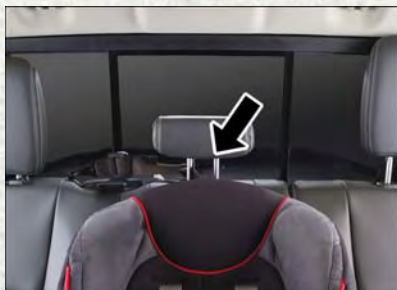
Tether Strap Through Center Tether Strap Loop
