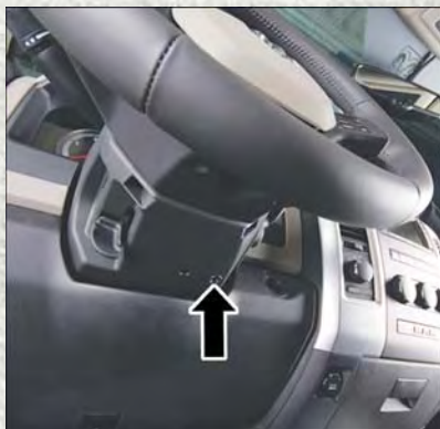
Shift Lock Manual Override Access Port
