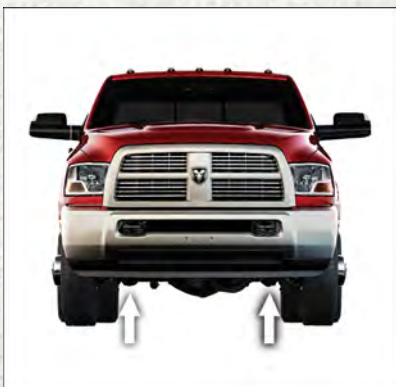
Front Jacking Location
