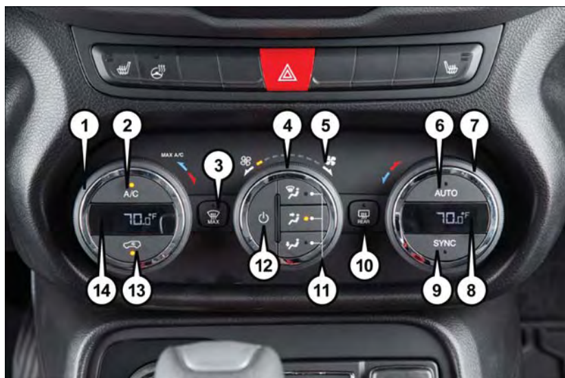
Automatic Temperature Controls (ATC)
