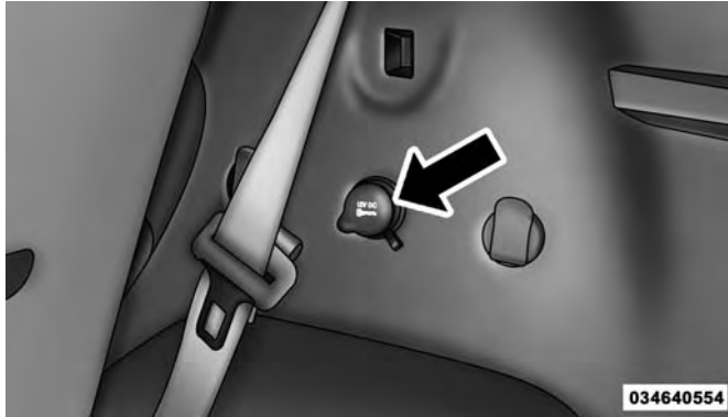
Rear Cargo Power Outlet
