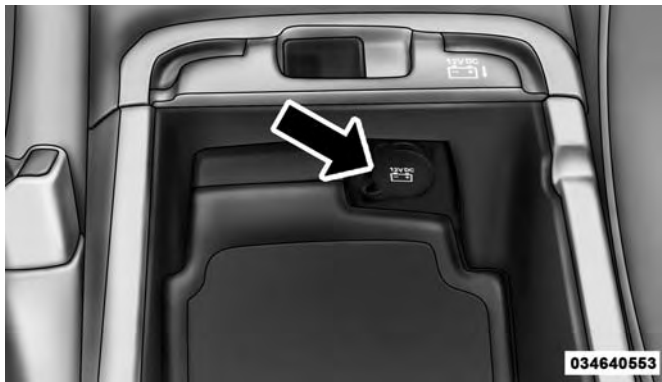
Front Center Console Outlet
