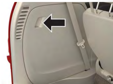
Jacking Equipment Location
