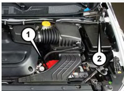
Positive Battery Post
