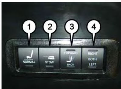
Rear Panel Power Switch Bank
