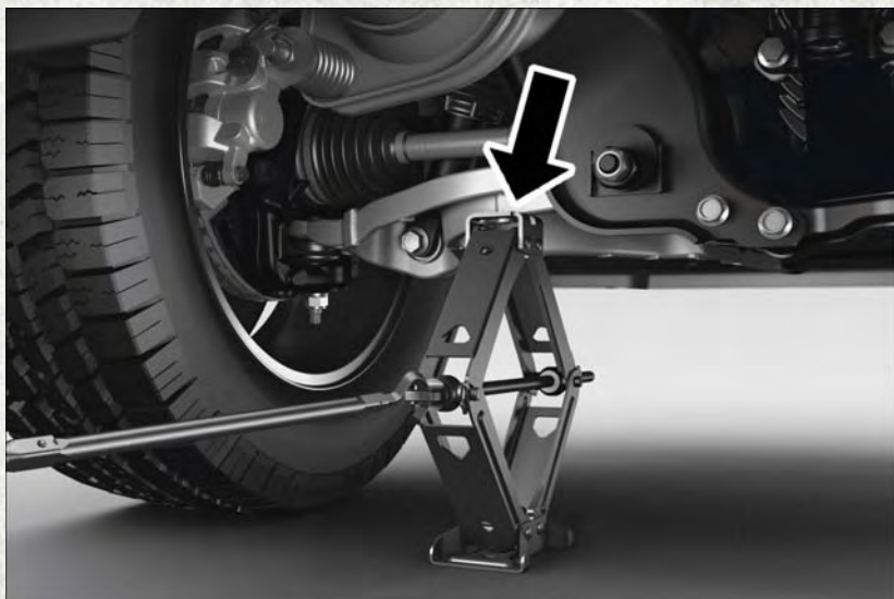
Front 4x4 Jacking Location
