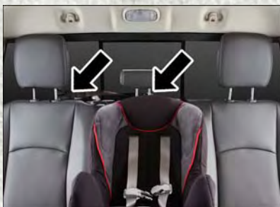
Tether Strap Through Center Tether Strap Loop And Attached To Outboard Tether Strap Loop
