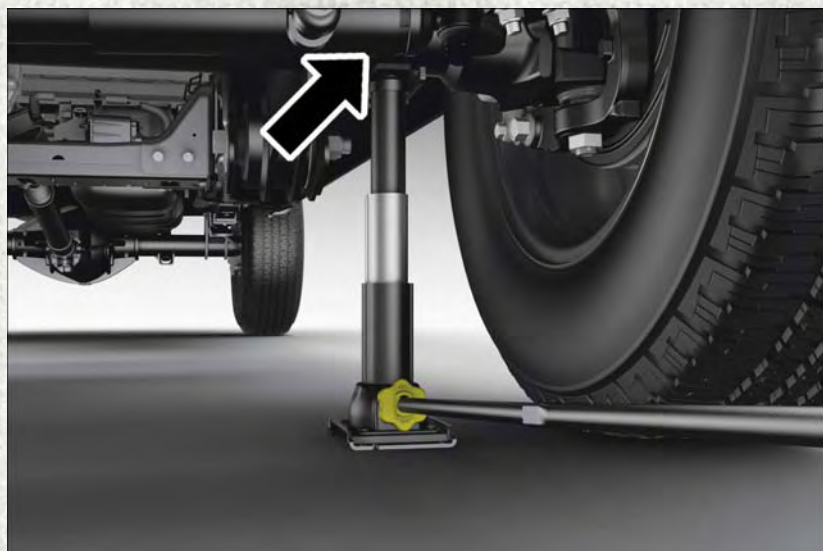
Front 4x2 Jacking Location
