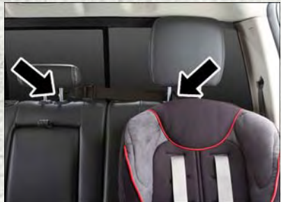
Tether Strap Through Outboard Tether Strap Loop And Attached To Center Tether Strap Loop
