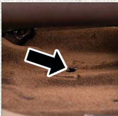
Floor Fastener Location
