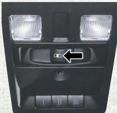
Power Sliding Rear Window Switch
