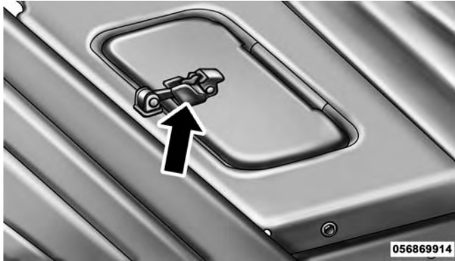
Manual Shut Off Valve Access Door
