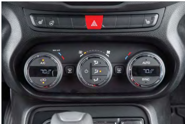
Automatic Temperature Controls (ATC)
