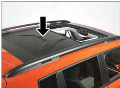
Installing Rear Panel
