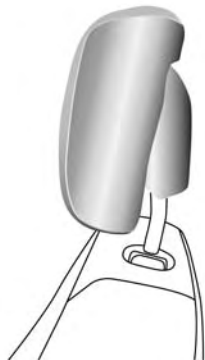
Active Head Restraint (Normal Position)
