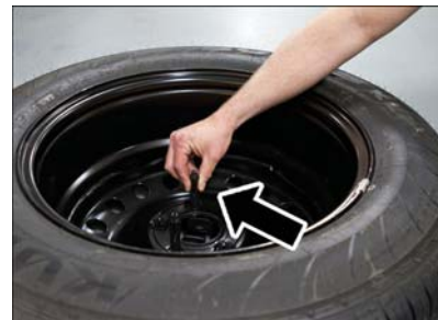
Protective Plate Removal
