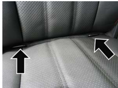
2nd Row Quad Seat LATCH Lower Anchorages
