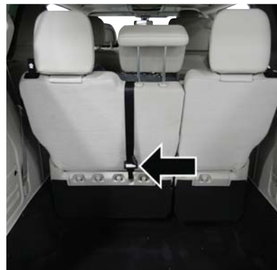
Tether Strap Anchorages (Third Row 60/40 Anchorage Shown)
