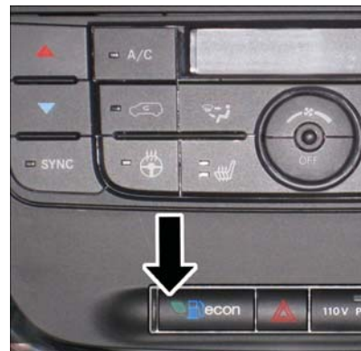
ECON Switch Location
