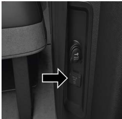
Power Inverter Outlet
