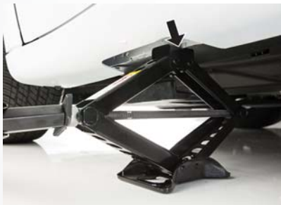
Front Jacking Location Engaged
