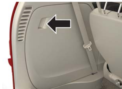
Jacking Equipment Location
