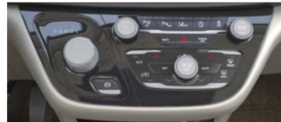
Automatic Climate Controls On The Faceplate
