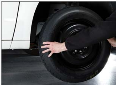
Installing Compact Spare
