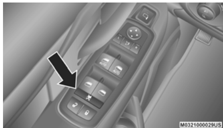
Window Lockout Switch
