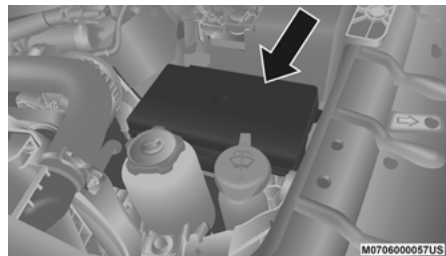
Power Distribution Center Location
