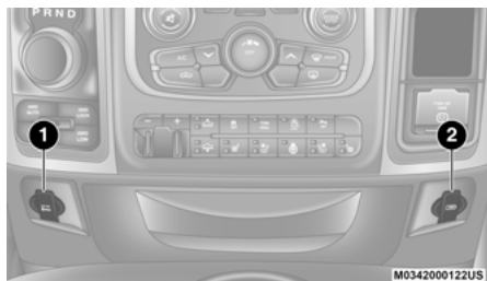
Power Outlets – Center Stack
