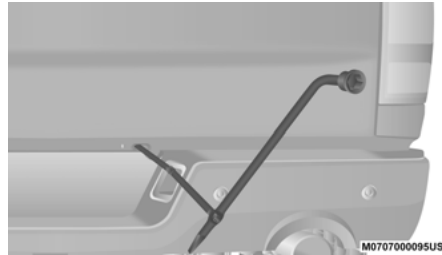
Inserting The Extension Tubes Into The Access Hole
