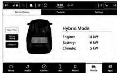
Power Flow Screen
