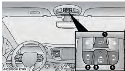
Overhead Console Power Switches
